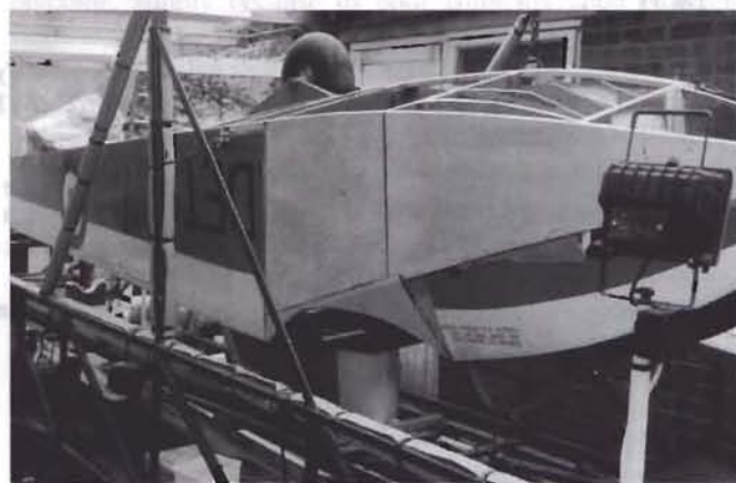
A later stage of the repair to the fuselage of the T21. Photo M. Powell.
