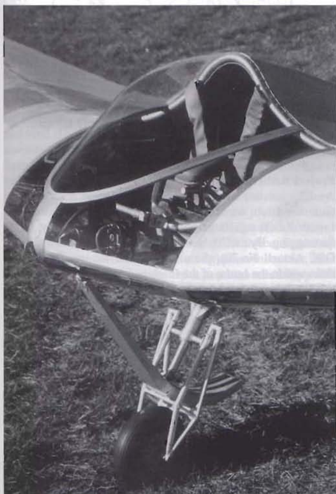
The centre section of LA-AD which was built from scratch by Peter Hanickel. The prone pilot's position and "handle bar" control stick can be clearly seen. Photo via Peter Hanickel.
