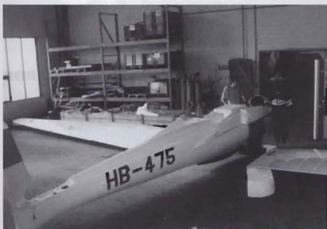
The Kranich 2B-1 HB-475 being rigged in the workshop for the first time after restoration. It was made by Kittelberger, Rheinau Höbert, near Breganz in 1943. Photo Werner Roth.
