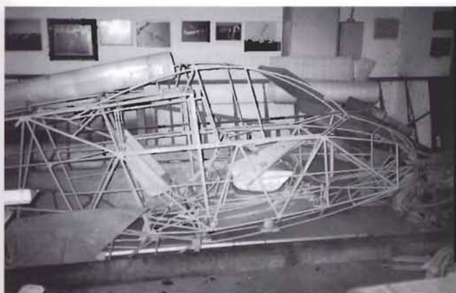
The on-going repair to the fuselage of the Grunau Baby V at Achmer. Photo Manfred Hermeling.
