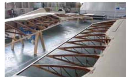
The wing of MG-19 ready for covering with new fabric.
