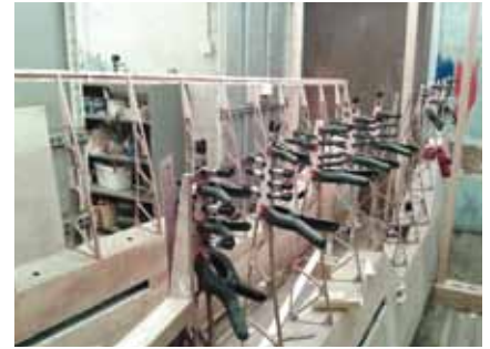
Buckminster Vintage Group EoN Baby (BGA 629) gets new trailing edges. Photo Bruce Stephenson
