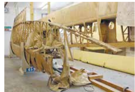
Although the fuselage was in good shape, the same could not be said if the port wing, as this photo testifies. Photo Paul Haliday
