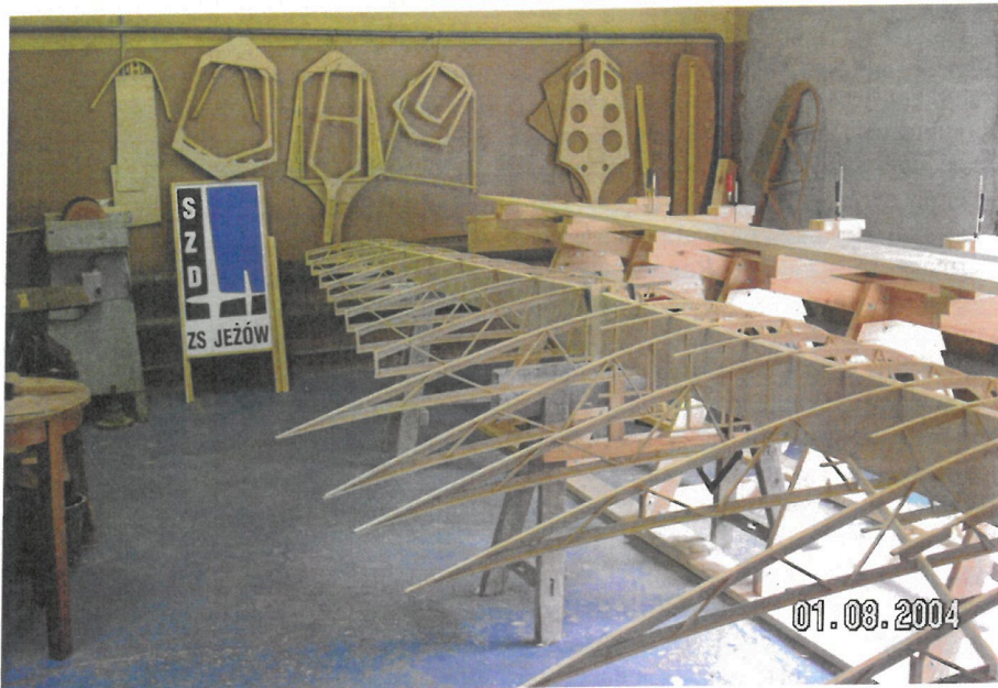
Above: wing of the Salamandra under construction in the SZD works at Jezow Below: VGC members inspect ailerons of the Salamandra during a tour from the Rally
